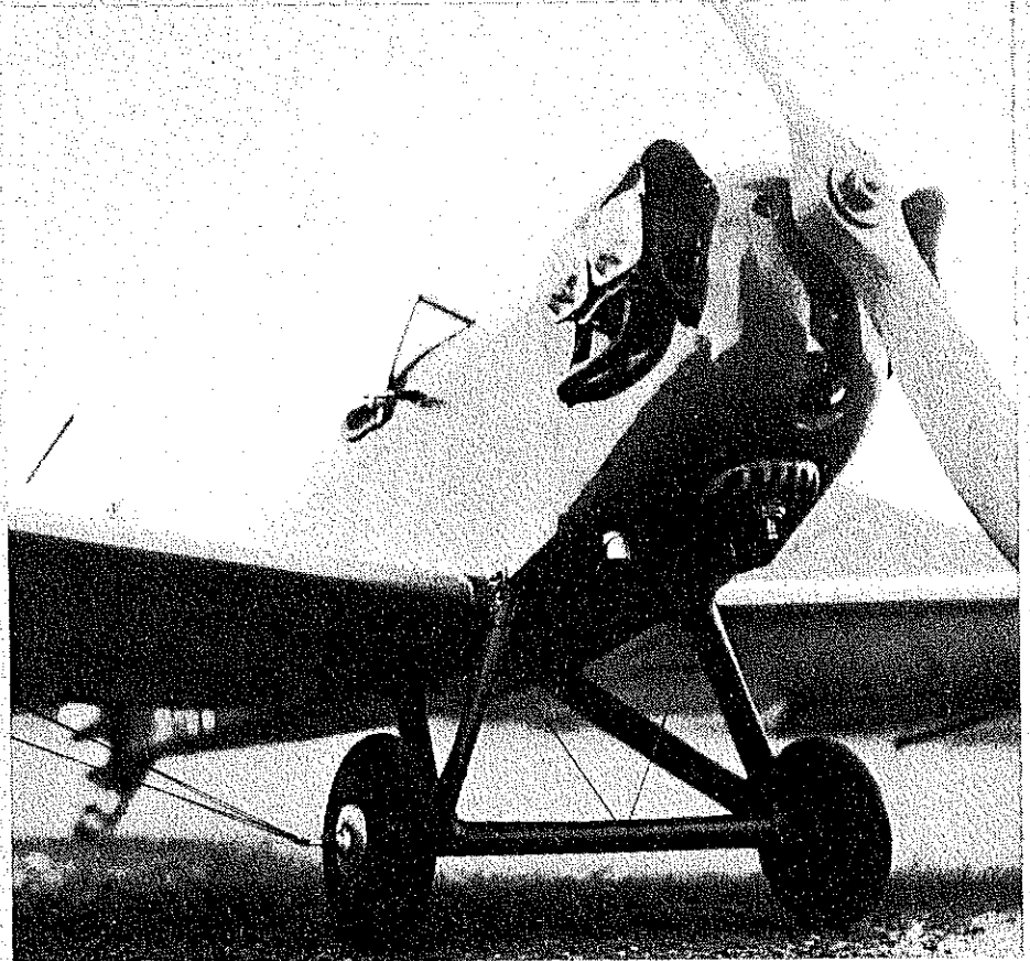
Flying (lift) wires attach to the landing gear axle as shown here. Note the exhaust manifolds and intake pipes, spark plugs and wires. A biplane Fly Baby homebuilt also is rather popular.
