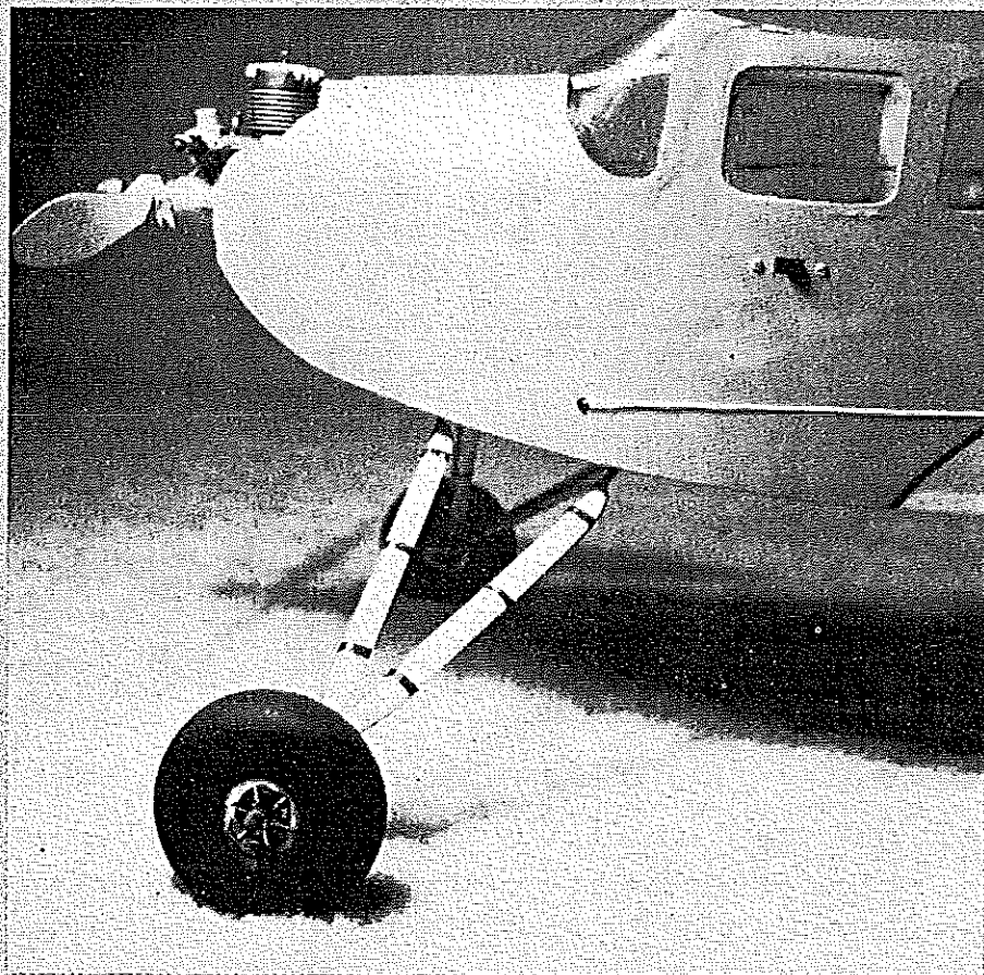
Because he wanted to reproduce faithfully the free flight structure, Emil used a built-in fixed landing gear, but typical, removable wire gear can be attached to ply plate with strap fittings.
