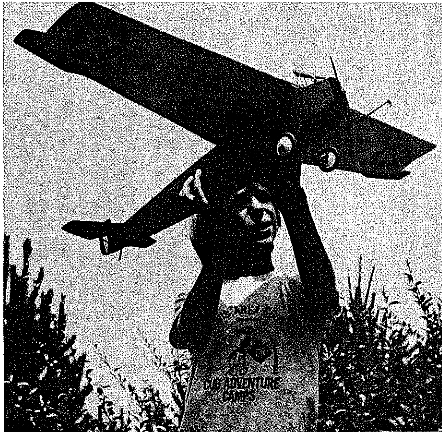
Andrew holding Dad's faithful copy of the historic Fokker. Although the tail surfaces appear tiny they are slightly enlarged from scale—for sport flying probably should be modestly enlarged again. Real cantilevered wing is said to have been enlarged from wartime Fokker D-VIII.
