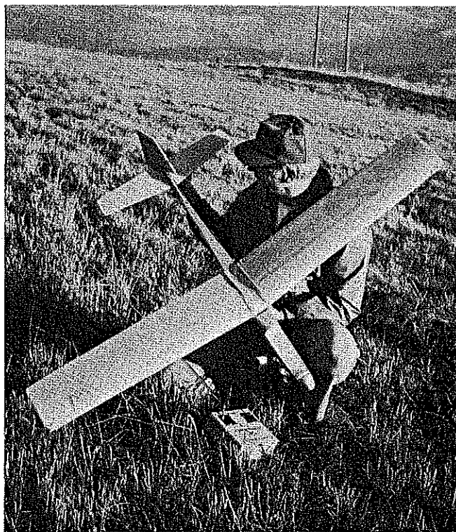
A rudder linkage adjustment brought about by the cold wind effects on nyrod pushrod guide transported to site in nice warm car.
