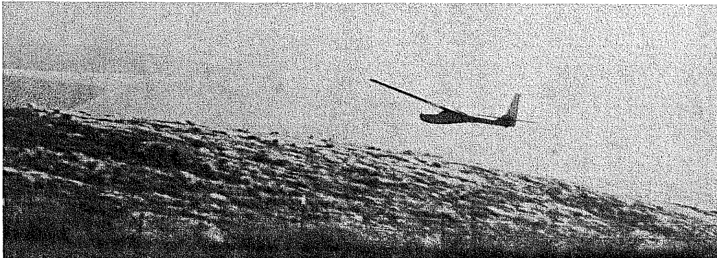
Beginning of another challenging flight. There is a slight ballooning tendency due to rising air—requiring slight down to avoid stall. The launching hand must be quickly diverted to the transmitter. Below: Low pass in front of flier. Turns should be away from hill until basic soaring techniques are mastered. Long gradual slopes like this one provide the smoothest air.
