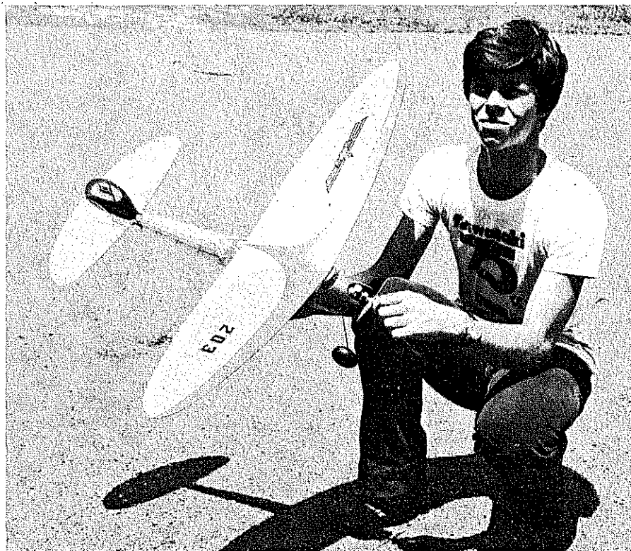
Murray's airplanes were distinguished by a not-often-seen wing design which had curved dihedral—rather like today's Hobbie Hawk sailplane—and an elliptical sheet-balsa planform.
