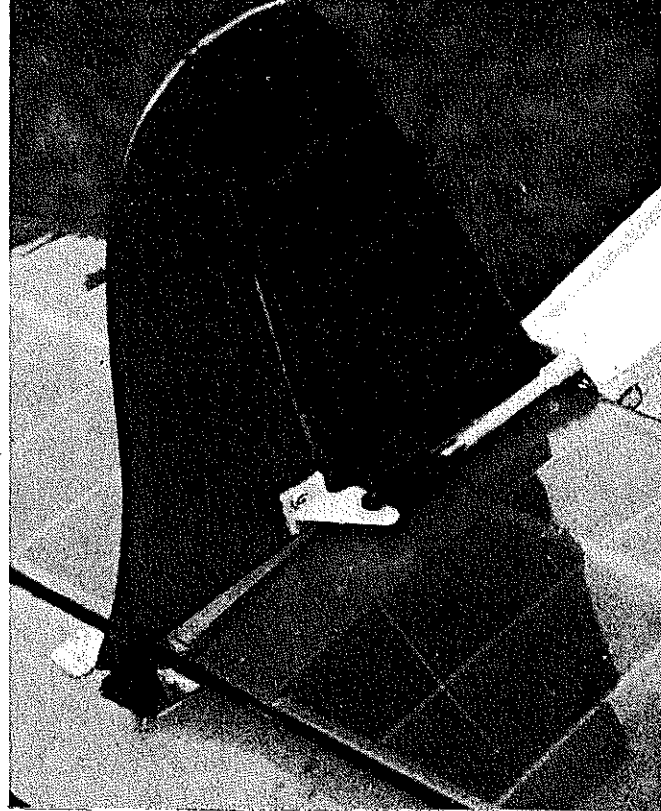
Details of the movable rudder and elevators on the RC-Assist version. Hole in elevator clears rudder when flipper is up. SAM rules require an .09 for Radio-Assist on this model.
