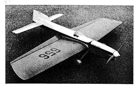
Purposeful and pretty, the model is displayed here with elevators and flaps displaced to 35 degrees—which is adequate. It's light construction contributes to tight turning ability. Although light, the model is strong.
