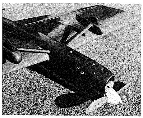
Moments and areas are typical of the all-out stunt machine. Slight rudder offset is used. No engine offset is required. Ship is adequately powered by a .35. The model is named after the Cardinals of North Idaho College.
