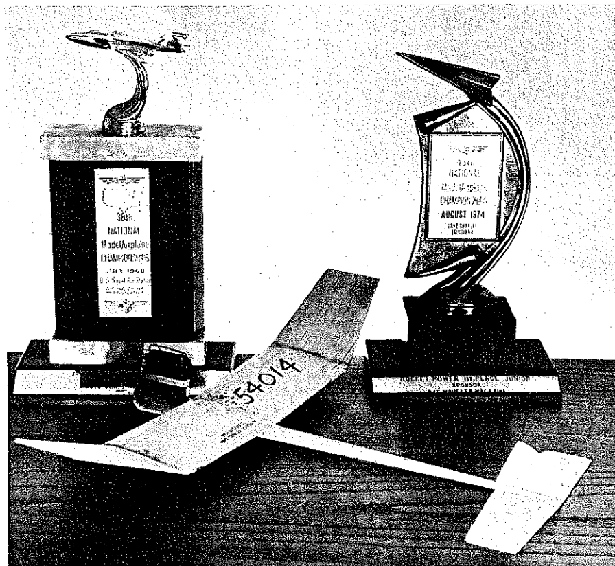
Hot Wood as built by young Greg Mills with the trophies won at the 1969 and '74 Nationals. The high thrust line eliminates any "power zooms."
