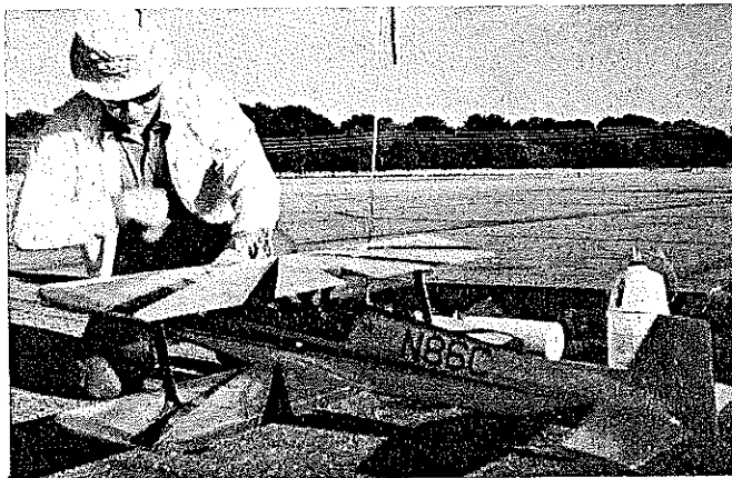
Left: Jerry firmly flips the 11-7 propeller. The ship was tested for structural integrity by dozens of straight-down flights through hundreds of feet of sky followed by a square corner. This simulated landing shot makes the point that landings can be quite slow without dropping a wing. It can be flared until the tail wheel touches.
