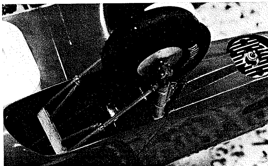
Although the complicated retractable landing gear—of course it works!—is fully detailed in both the text and on the plan, there's nothing like a picture to help clarify things.
