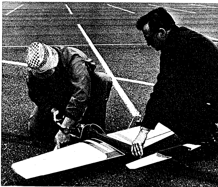
Bob Emmett holds for Don Schultz. Model is FAI Avenger, OS 35, 47 oz. on a span of 57 in.
