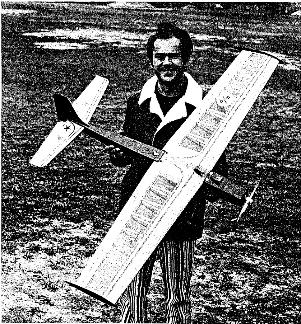
Builder of the prototype was Greg Malinowski, who poses here with the Electric One. The transparent Solar Film covering shows off the light-weight construction techniques. Greg went so far as to make cut-outs in the wing ribs and tail surfaces. He went all out, selecting light balsa, keeping the use of glue to a minimum. Throttle servo was linked to a small switch for on-off control. He used equipment with its smallest servos.
