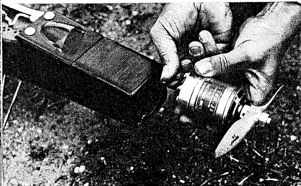
Above: Weight of battery packs calls for unusual radio equipment location, accessible through hatch—also balances model. Below: How motor is installed and removed, by tight friction fit into rolled thin plywood tube epoxied into fuselage. Wire connectors plug onto rear of motor.
