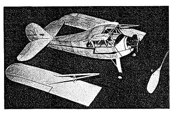
Top: When it was new—now 5-1/2 years old—the K was an ultra light-weight good for 90 seconds. Left: By assembling-struts to each half wing, panels can be quickly attached or removed for travel. The details show clearly in photo directly above, as does center section construction with two dowel ends jutting from each side to slide into wing holes. Model in pix is rebuilt after another in-flight model fell on it. It is lightly doped in yellow with black trim lines. (Photos by John Sites.)
