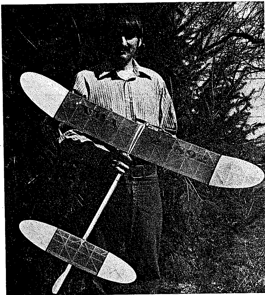
Contrasting colors of covering material make for a pretty airplane. Jap tissue is given three of thinned clear dope, and a final of K&B epoxy clear paint—stands up to high-nitro fuels. Curved portions of all tips and stab edges are built up from 1/16 x 1/8 laminations.
