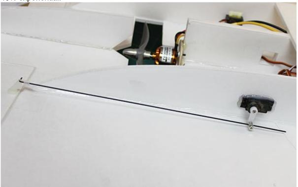
Servo Installation The servos are hot glued in place and the control horns are glued in place using foam-safe CA. A Dubro mini-keeper is used to lock the pushrods to the control horns.
