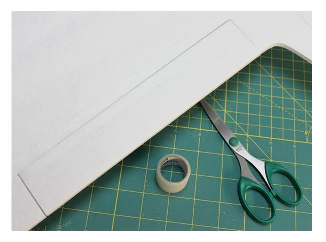
The top of each elevon is hinged with a strip of Blenderm tape across the full length of the piece.
