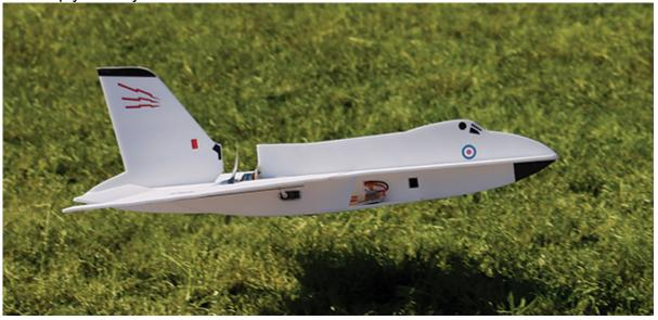
The Vulcan's glide is slower than walking pace with no tendency to tip stall. Note the nose-up angle of attack and the position of the elevons as it sets up for a landing.
