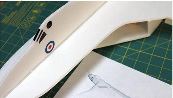
Markings for this version of the Vulcan are minimal. The cockpit markings are from a MonoKote trim sheet and the RAF roundels were printed and attached with Elmer's spray adhesive.
